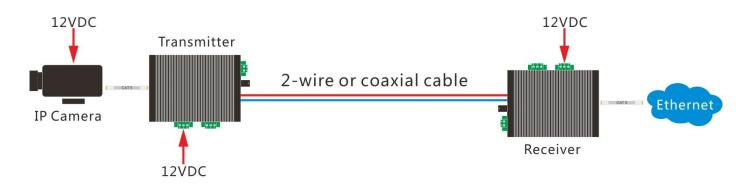
**Notes:** In order to ensure the power supply with low transmission loss, we suggest using high quality cables such as coax cables above RG59, 2-wire cable above 2×0.75mm<sup>2</sup>, network cable above Cat5.
