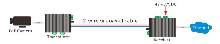
3. If the remote devices are not PoE devices, you can offer 12VDC power supply for the Receiver and Transmitter unit separately; the remote devices need to be powered separately.
